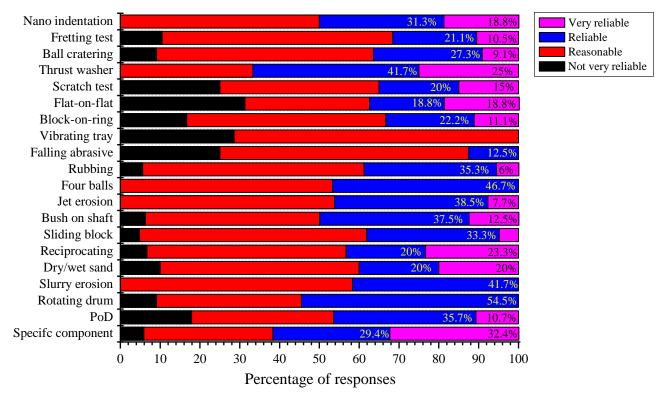
Figure 17 The quality of data from tribological testing
