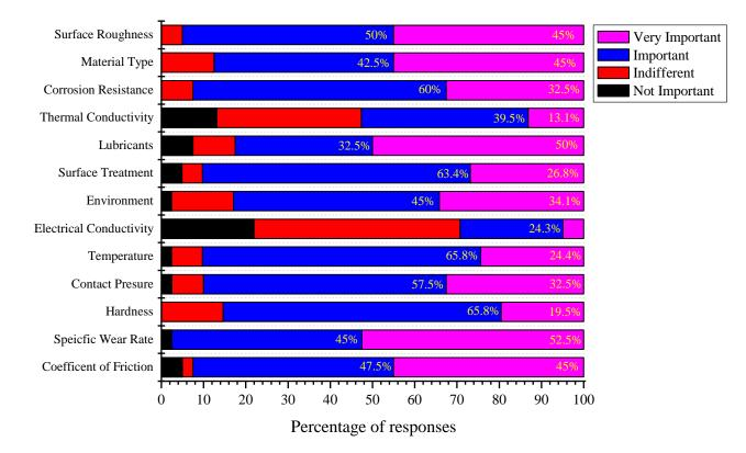
Figure 10 Importance of factors in designing tribological components
