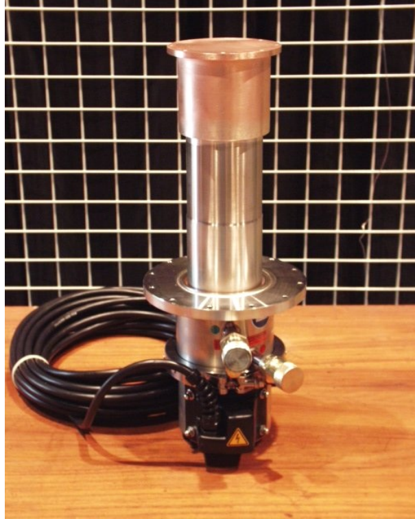
FIGURE 3.2: Leybold coldhead RGS120T (reproduced from [8]).
