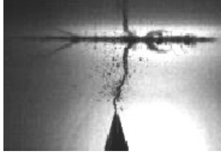
FIGURE 2.1: Cathode filamentary streamer in LN 2 at 77.5 K, atmospheric pressure, 26.4 kV AC (reproduced from [10]).
