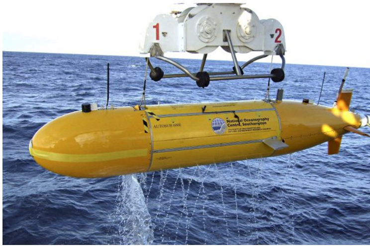
Figure 2.3: Autosub6000 being recovered onto the RRS James Cook. Note the location of four control surfaces and a propeller at the rear of the vehicle.
