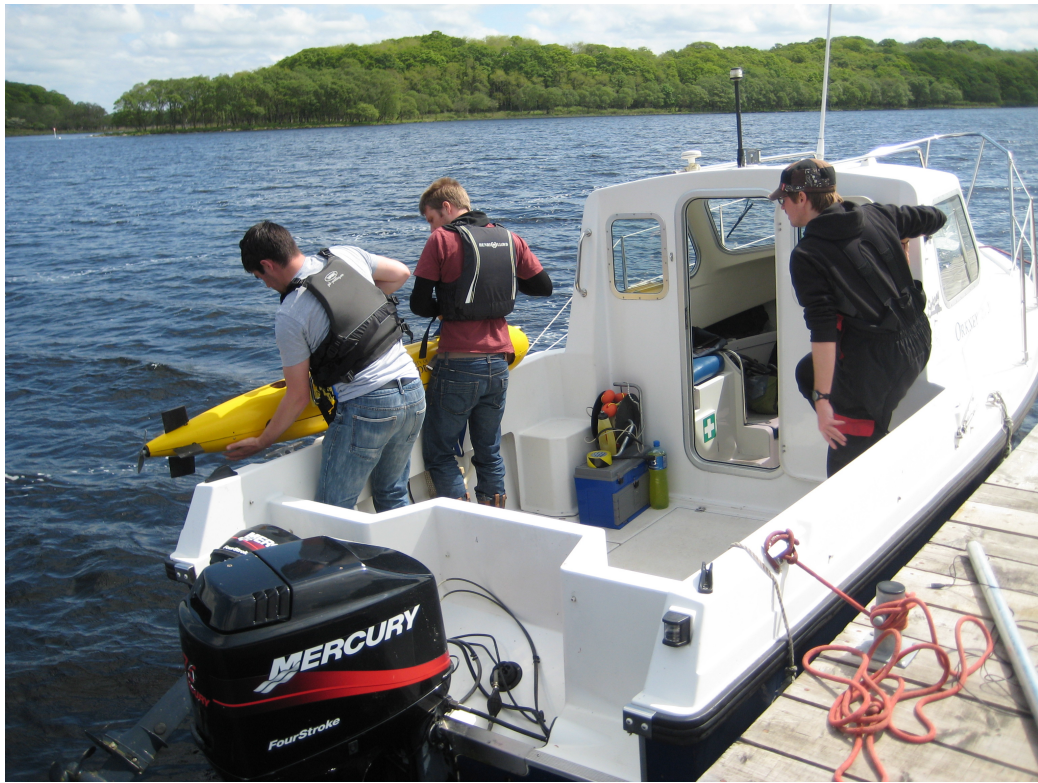
Figure B.4: Delphin2 AUV being launched off the side of the AFBI boat at Carrickreagh Bay.
