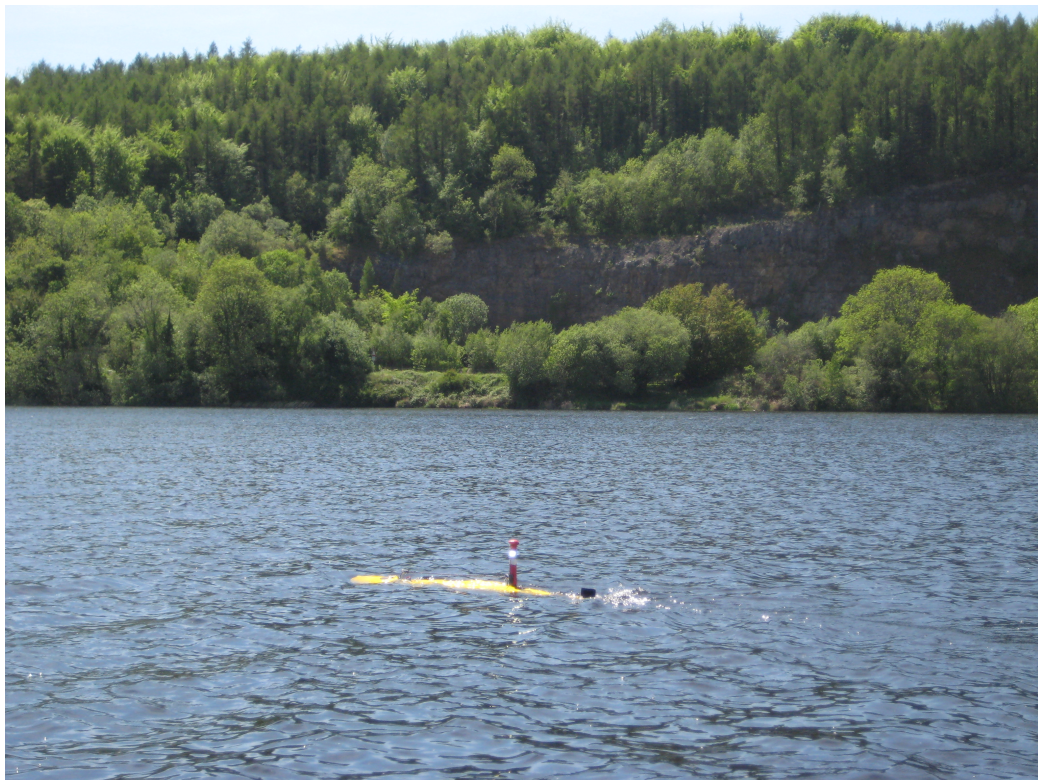
Figure B.5: Delphin2 AUV returning to the jetty in Carrickreagh Bay after a successful video survey of the lough bottom.
