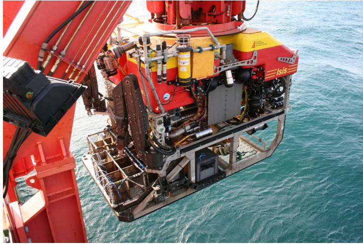
Figure 2.1: Launching of ROV Isis from RRS James Cook. Note the two manipulator arms in the folded position and the various lights, cameras and thrusters.
