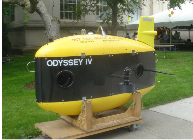
Figure 2.4: Odyssey IV AUV. This vehicle has the ability to hover and transit at up to 2.0 m/s. Picture courtesy of MIT.
