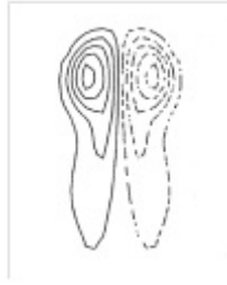
Figure 2.6: Head-Tail structure from Kida et al. (1991) vorticity contours on the symmetry plane. Solid and broken lines represent vorticity of opposite signs
