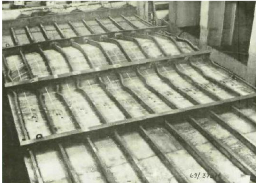
Figure 4.7 – Smith [67] Grillage Experiment Case 3a Failure Condition
