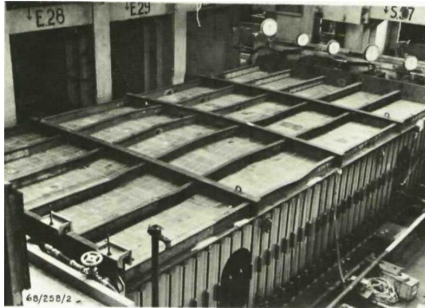
Figure 4.11 - Smith [67] Grillage Experiment Case 5 Failure Condition
