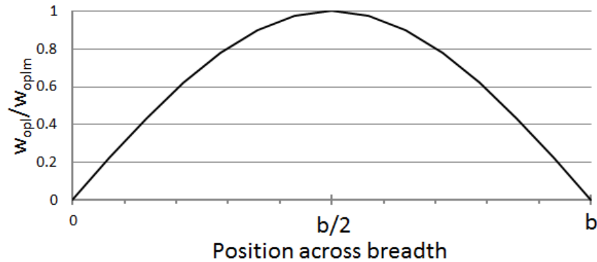
Figure 2.17 - Example plate imperfection shape across breadth between longitudinal stiffeners at a/2
