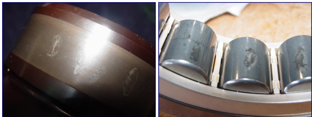
Figure 3.11: Case 4 - Photos showing damage to aft bearing inner race and rolling elements
