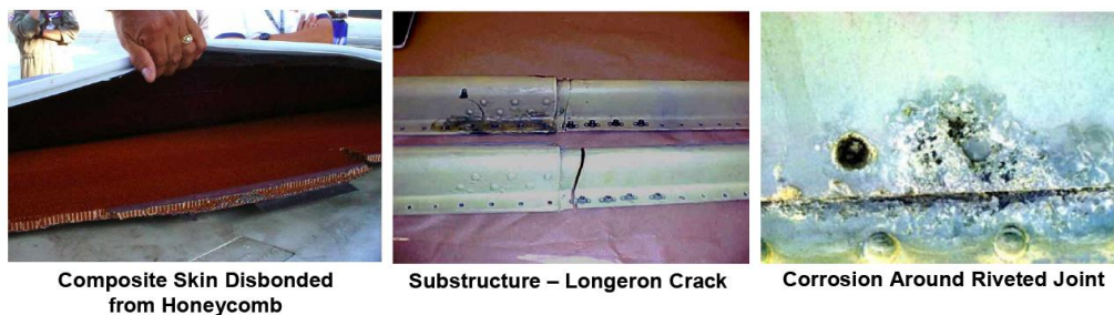
Figure 2.4: Examples of disbond, crack and corrosion damage, [32]
