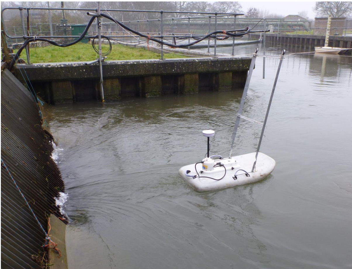
Figure 4.6 Raft-mounted Acoustic Doppler Current Profiler (M9 RiverSurveyor, SonTek) attached to transect guide line
