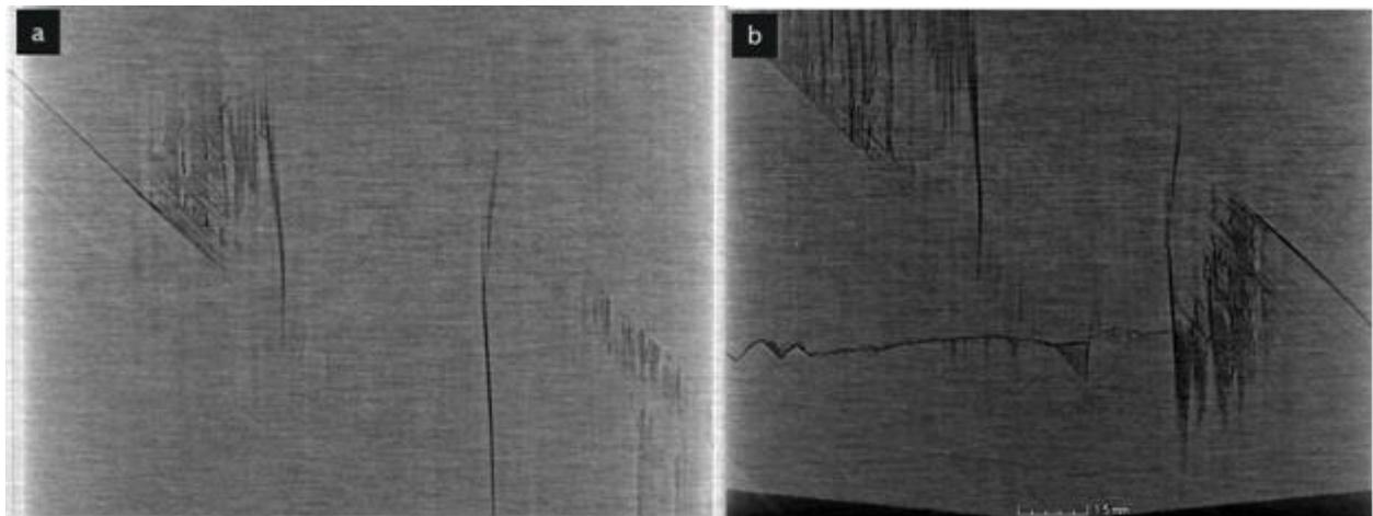
**Figure 8.** In-plane  $\mu$ CT slice showing a  $0^\circ/45^\circ$  ply interface a) damage after impact and b) micro-buckling occurring at 99% of failure load for a particle toughened system
