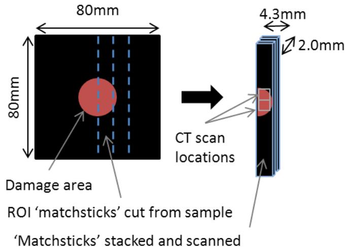
**Figure 2.** ‘Matchstick’ sample preparation across damage areas for CT analysis
