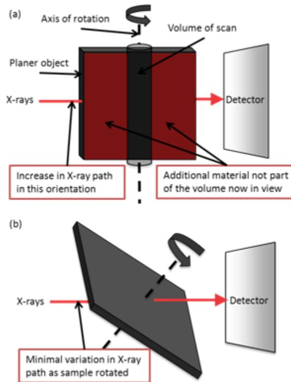
**Figure 1.** Schematic comparison of geometries associated with: (a) SRCT and (b) SRCL
