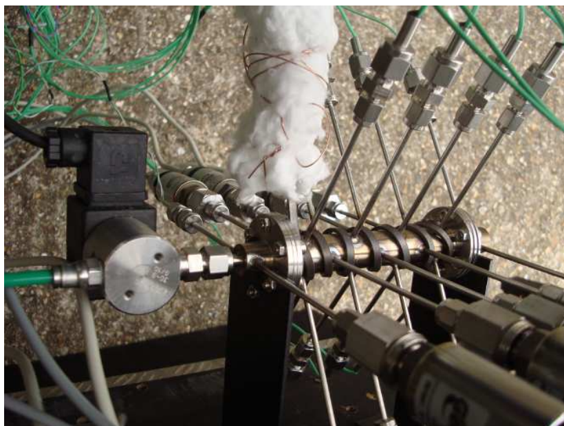
Figure 5.3: Instrumented catalyst bed used for validation
