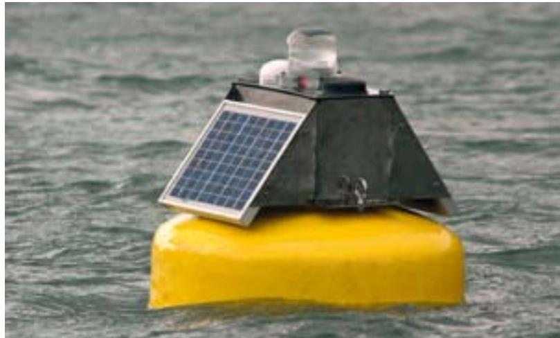
Triskel Marine's DataBuoy is a cost effective way of monitoring the inshore marine environment in real time. The buoy is tough, light weight, easily deployed, and completely autonomous, with the following specifications:
