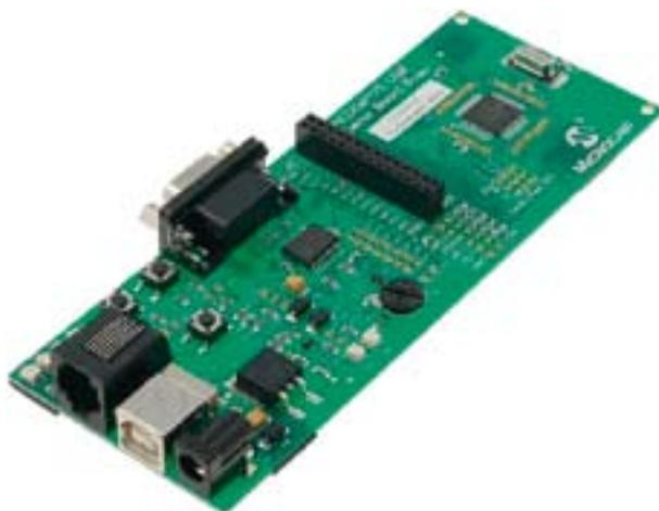
When attached to an USB port, the SSA allows the DAS to download its configuration data. In a next step, the DAS uses this information in the similar way it would use the configuration data obtained from the 'sensor types' database. Finally, the SSA switches to the 'transparent' mode and allows direct communication between the SensorSA DAS and the SSA RS-232 interface.
