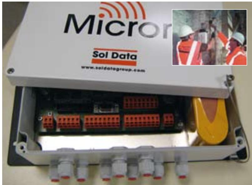
The Micron smart sensor nodes have an integrated battery, which allows a guaranteed autonomy of 2 years. This autonomy may vary depending of the sensors attached and the frequency of measurements. An external power source can be connected, so e.g. photovoltaic panels could also be deployed to power the sensor nodes, and take over the battery powering.
