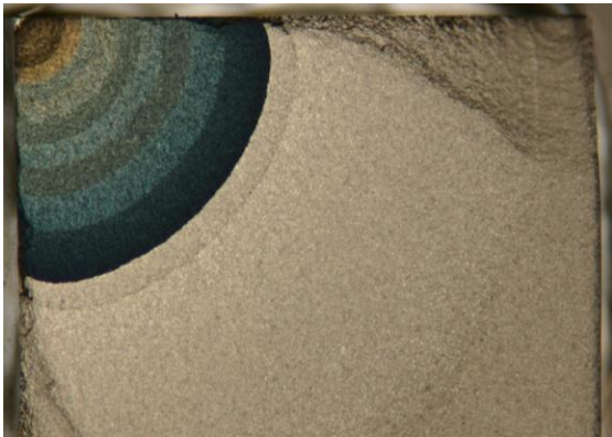
Figure 6-26: Fracture surface of CNT test carried out in air at 400 and 650°C (more details in Table 17) (sample CC013)
