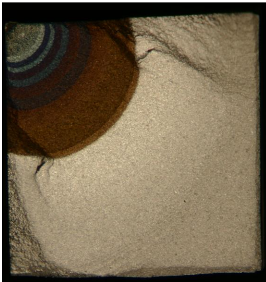
Figure 6-32: Fracture surface of CNT test carried out in air at 260 and 540°C (more details in Table 17) (sample CC001)
