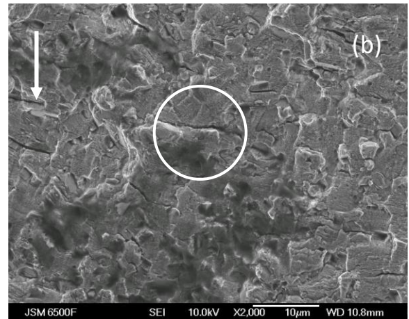
Figure 5-6: Fracture surface of U720Li FG PM at 300°C in air \Delta K_i=17.7\text{MPa}\sqrt{\text{m}} in the Terraced region at c=5.2\text{mm} and an estimated \Delta K\approx 42\text{MPa}\sqrt{\text{m}} (Arrow indicates crack growth direction, circle shows secondary cracks) (a) at low magnification showing the flat and deflected terraces (b) At higher magnification showing stage II growth in the flat region with sliptraces and secondary cracks merging over several grain sizes
