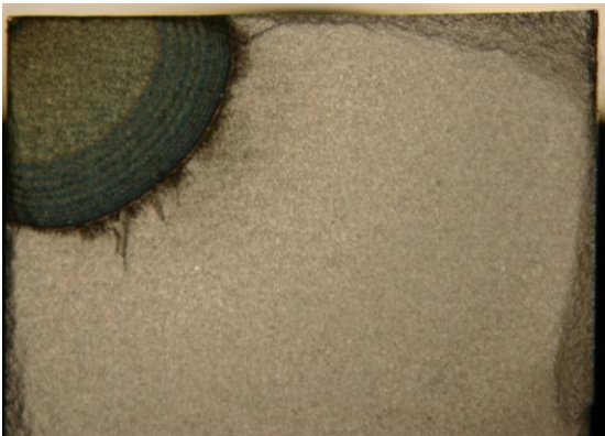
Figure 6-27: Fracture surface of CNT test carried out in air at 650 and 400°C (more details in Table 17) (sample CC012)
