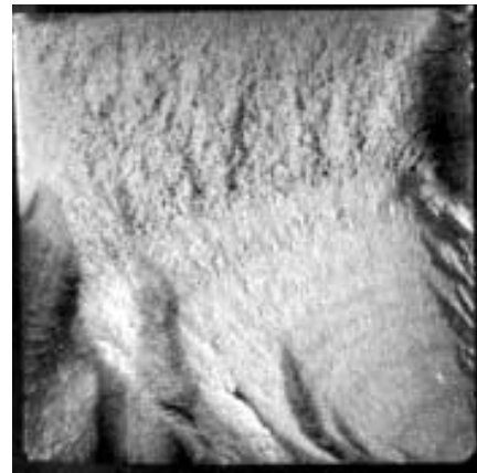
Figure 2-9: TDC fracture surface with Beachmarking showing shear lips form progressively during fatigue [4]
