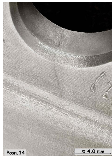
Figure 6-62: Deflected crack on disc air hole (number 14) failure initiated from the chamfer [101]
