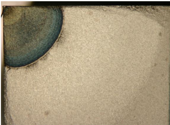
Figure 6-28: Fracture surface of CNT test carried out in air at 650 and 400°C (more details in Table 17) (sample CC014)
