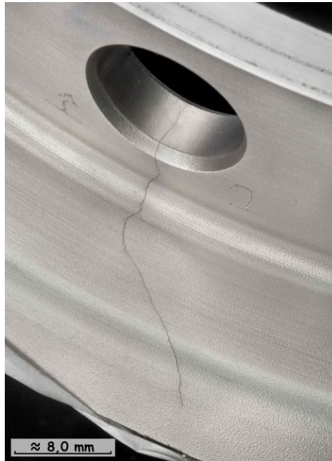
Figure 6-60: Deflected crack on disc air hole (number 2) failure initiated from the chamfer [101]
