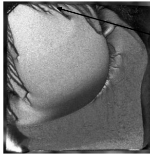
Figure 5-62: Fracture surface of U720Li PM FG with \Delta K_I=17.7\text{MPa}\sqrt{\text{m}} at 300^\circ\text{C} in air
