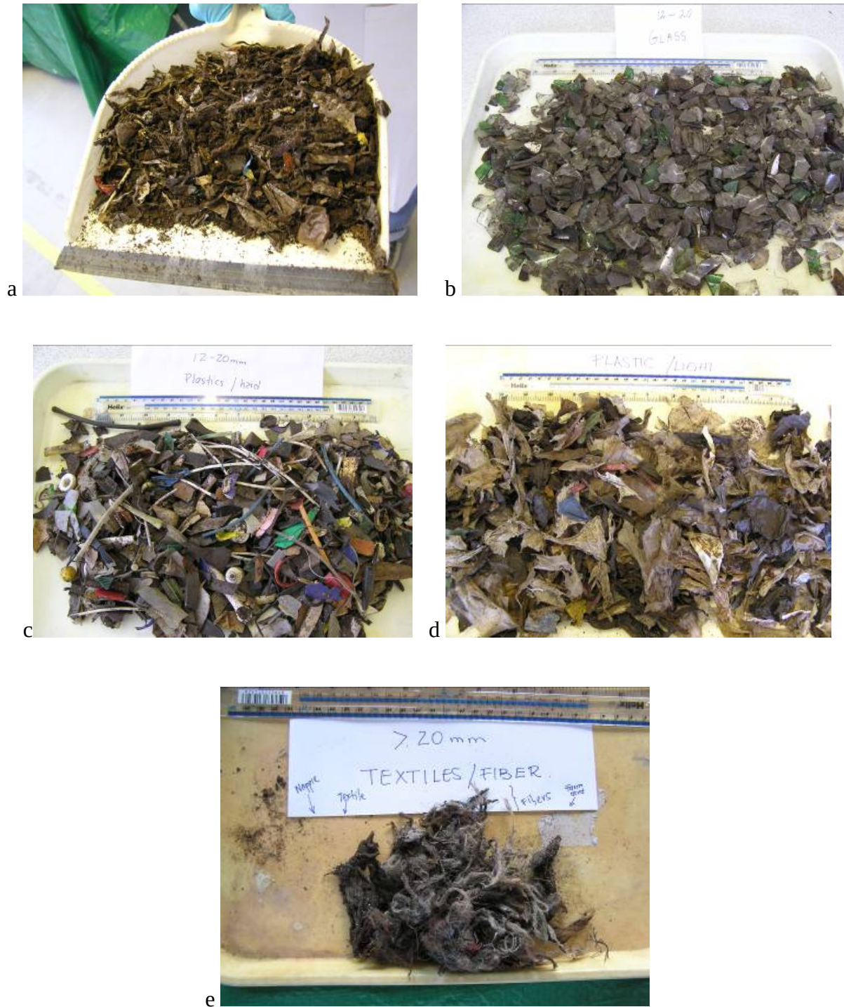
Figure 6. MBT waste (a) before sorting; and after manual sorting: (b) “Glass” with size 12-20 mm; (c) “Rigid plastics” with size 12-20 mm; (d) “Flexible plastics” with size bigger than 20 mm; (e) “Textiles” with size 12-20 mm
