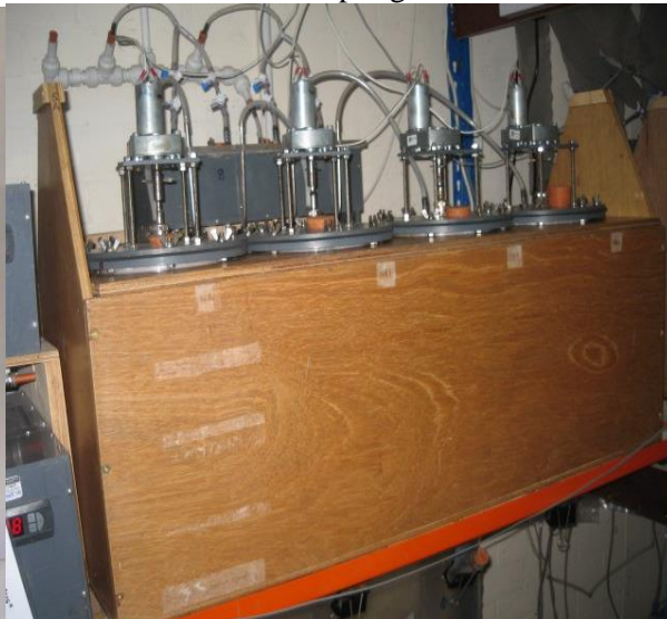
Figure 3. Set of 5 l digesters in temperature controlled housing
