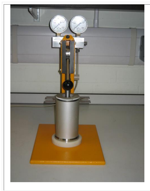
Figure 3.1 Photograph of the small capacity pressurisation unit and filling station
