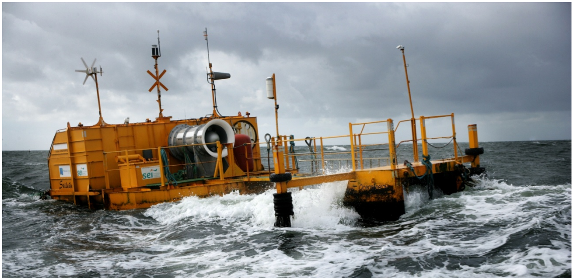
Figure 3.2, Reduced scale OE Buoy device being tested in Galway Bay [Source: Ocean Energy Ltd]
