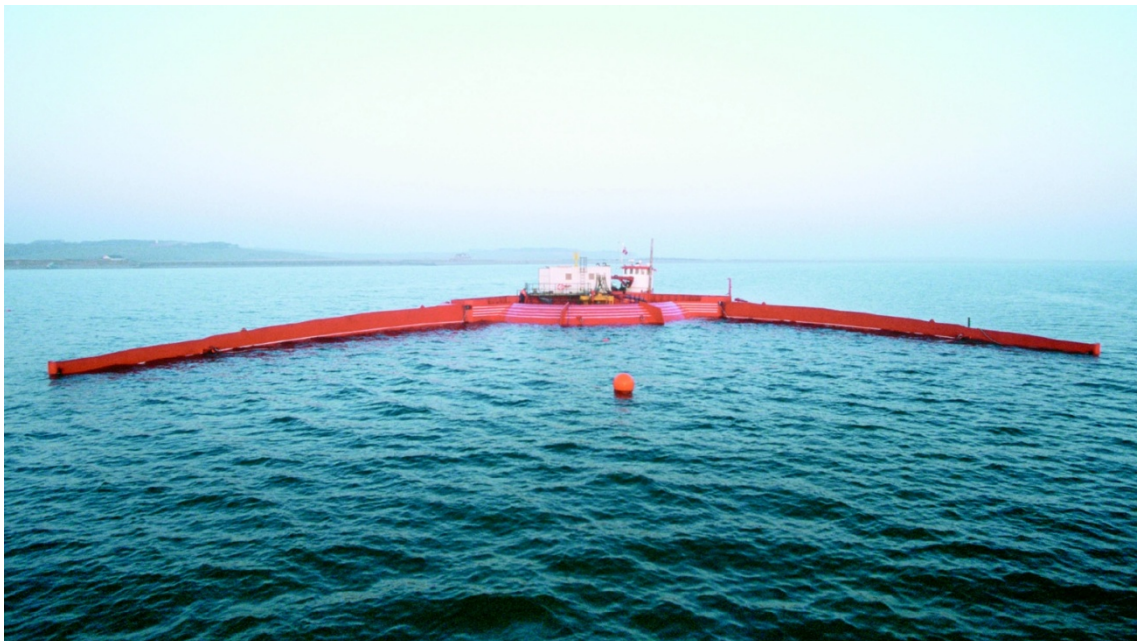
Figure 3.8, The quarter scale Wave Dragon prototype under test at Nissum Bredning [Source: Wave Dragon ApS.]
