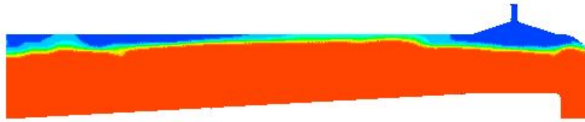
Figure 3.13, An example of a 1:10 scale CFD simulation showing the water volume fraction of a wave propagating along the duct.
