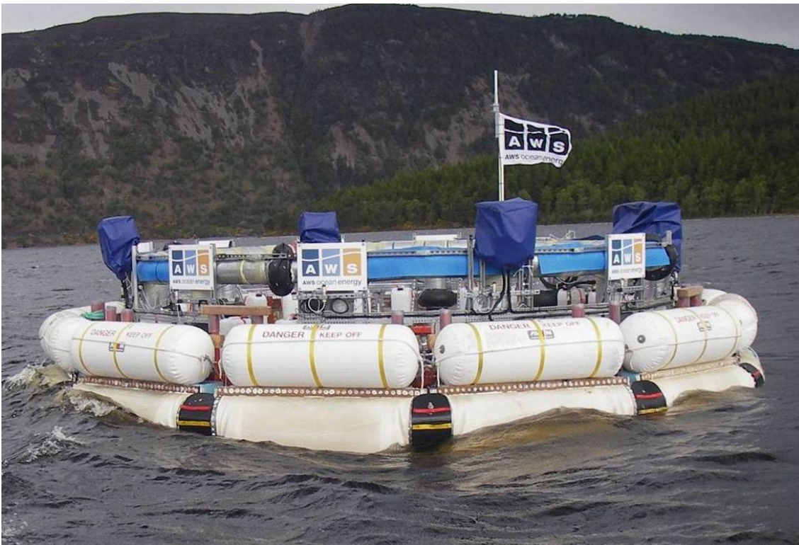
Figure 3.7, AWS's 1:9 scale device being tested in Loch Ness [Source: AWS Ocean Energy Ltd.]
