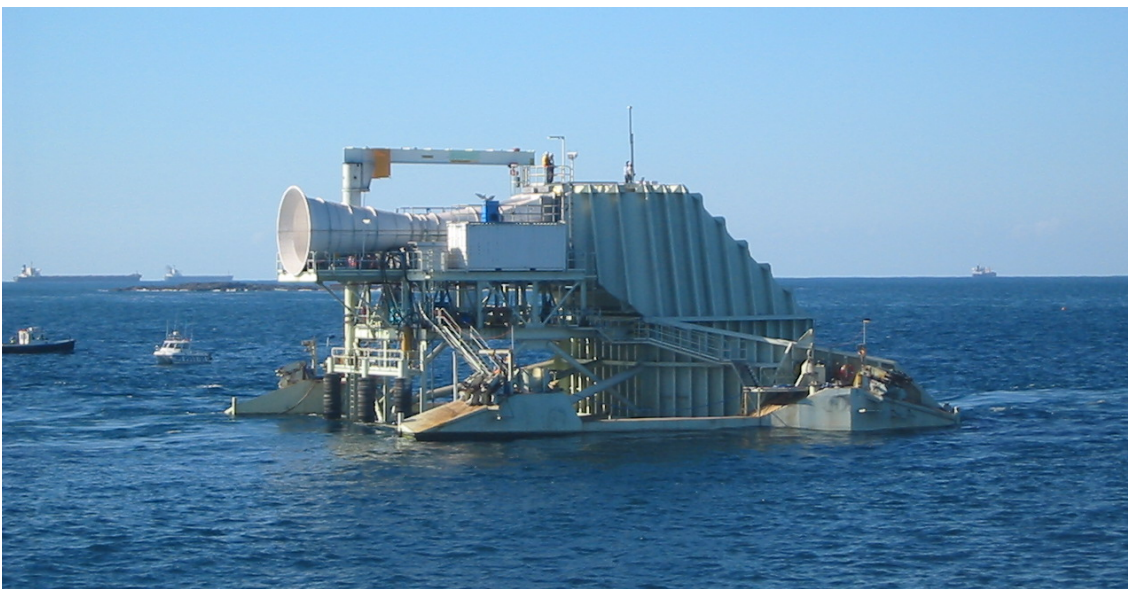
Figure 3.1, The Oceanlinx demonstrator with the collector on the right side of the device and turbine exit on the left [Oceanlinx]
