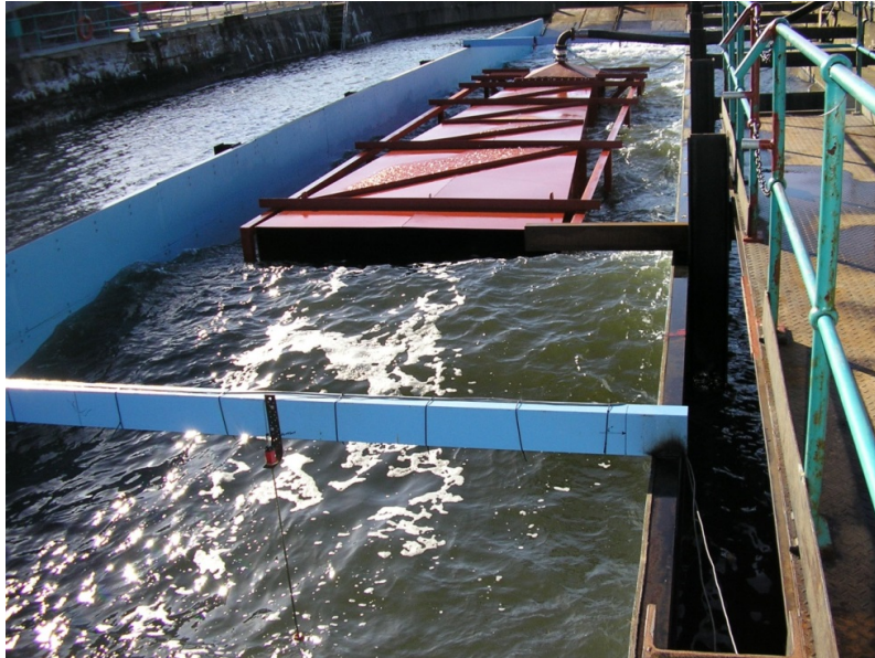
Figure 3.12, The 1:10 OWEL model under test in the wave tank at Narec in 2003.
