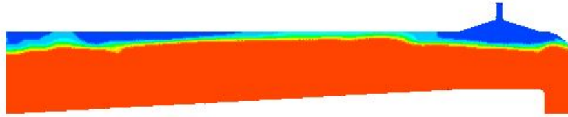
Figure 11.5, An example of a 1:10 scale CFD simulation showing the water volume fraction of a wave propagating along the duct.
