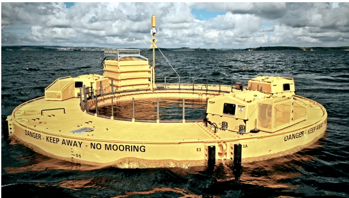
Figure 3.5, Fred Olsen's BOLT "Lifesaver"™ device installed at Fab Test, UK [Source: Fred. Olsen Ltd.]
