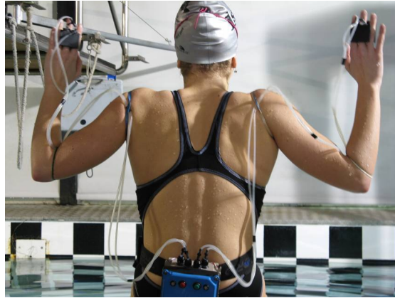
FIGURE 2.2: APLab’s KZ system for measuring pressure on swimmer’s hands 1 .
