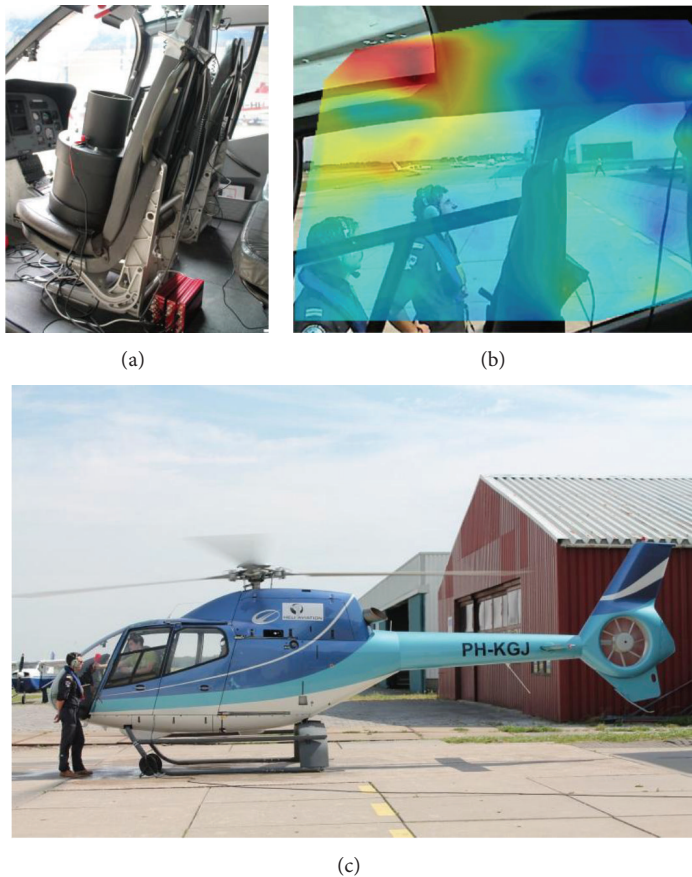
FIGURE 12: Pressure contribution mapping of a helicopter cabin interior between 180 and 250 Hz with a 10 dB dynamic range [12].
