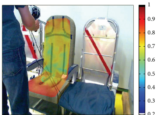
FIGURE 13: Local sound absorption mapping of a plane seat.
