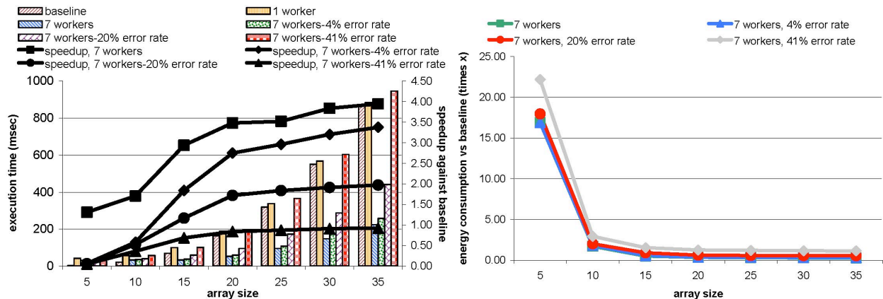
Figure 6 – Task-re-execution in the presence of faults: The matrix tree-multiplications micro-benchmark execution time and speedup (left), and energy consumption (right) against the baseline system.
