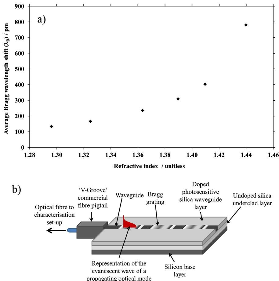
**Fig. 1.** (a) Calibration curve of a Bragg grating refractometer device to changes in refractive index and (b) an illustration of the Bragg grating refractometer devices used within this work.
