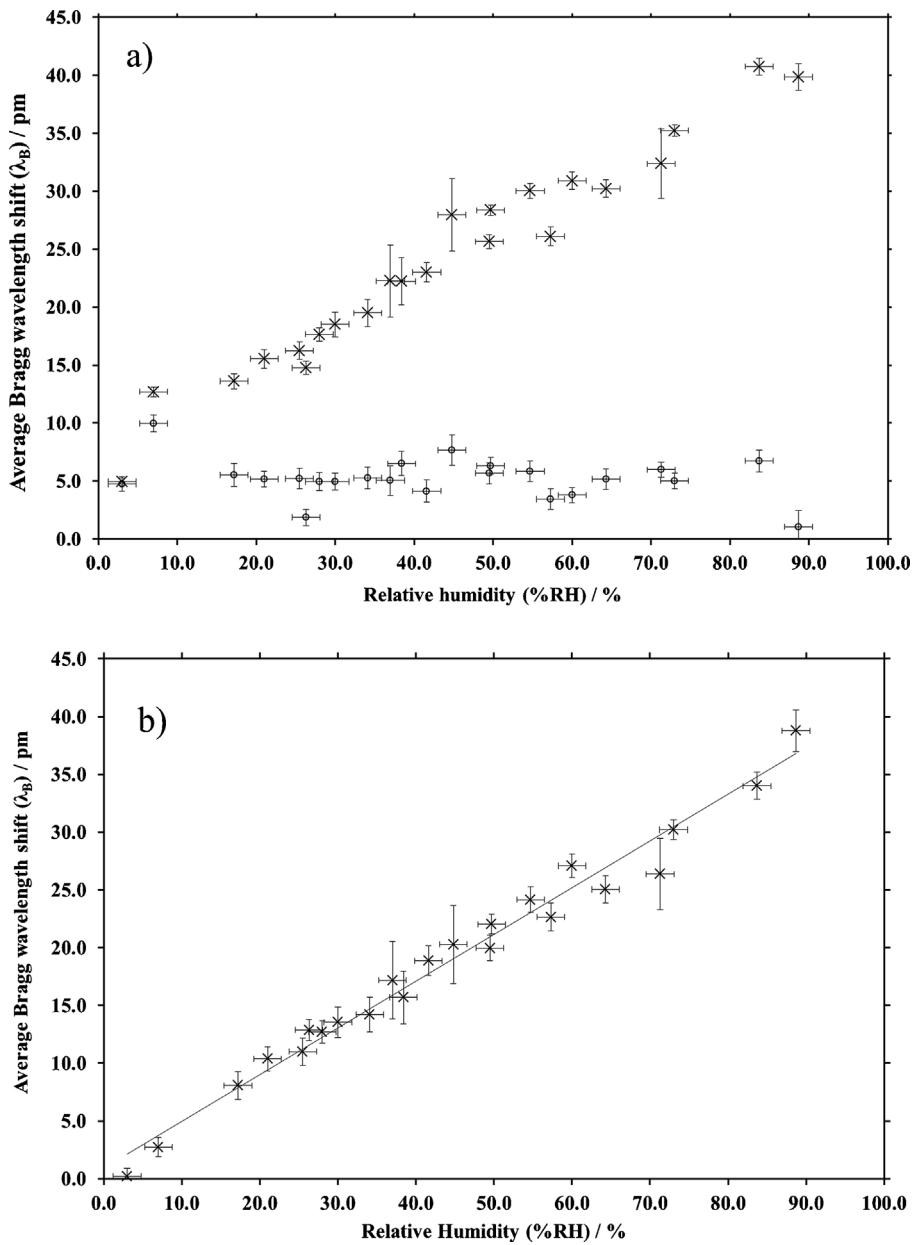
**Fig. 4.** (a) The average Bragg wavelength shift of the mesoporous silica sol–gel thin film region (crosses) increases when exposed to increasing relative humidity, %RH. In contrast the two uncovered Bragg gratings (circles) show no response to humidity change. (b) After subtraction of reference gratings an improved linear response to increasing relative humidity was observed, demonstrating on-chip thermal compensation.
