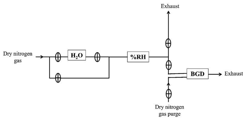
**Fig. 2.** A schematic of the gas flow network used to investigate the Bragg grating response to changes in humidity. Water vapour was generated by bubbling dry nitrogen gas through a de-ionised water reservoir ('H<sub>2</sub>O'). '%RH' represents the electronic reference hygrometer and 'BGD' is the location of the flow cell containing the integrated optical Bragg grating device. A second nitrogen purge was used to maintain a dry atmosphere between measurements.
