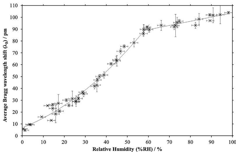
**Fig. 5.** Three data sets were collected from 0–100%RH after prolonged exposure to elevated humidity (>95%RH). Lines are guides for the eye only.
