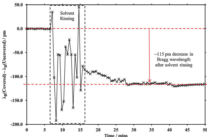
**Fig. 7.** The decrease in Bragg wavelength upon rinsing the contaminated aluminosilicate thin film Bragg grating hygrometer with methyl ethyl ketone (MEK) indicated the removal of surface contamination. The sharp jumps in refractive index within the hashed region correspond to individual solvent washes.
