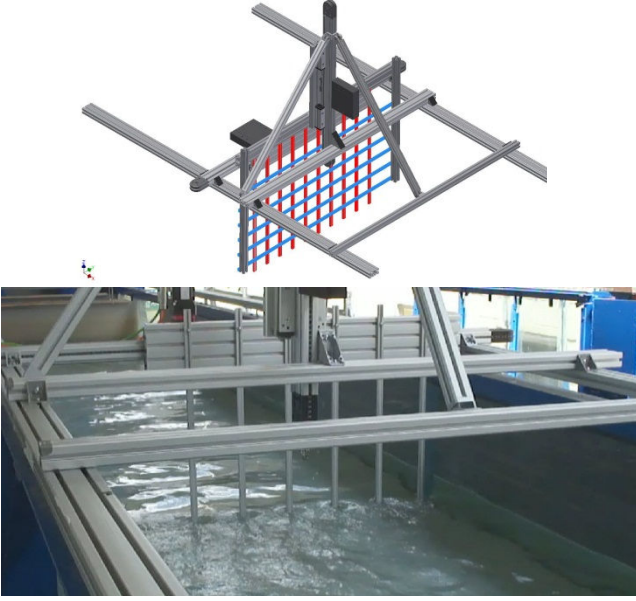
Fig. 2 CAD assembly and image of turbulence generator operating in flume
