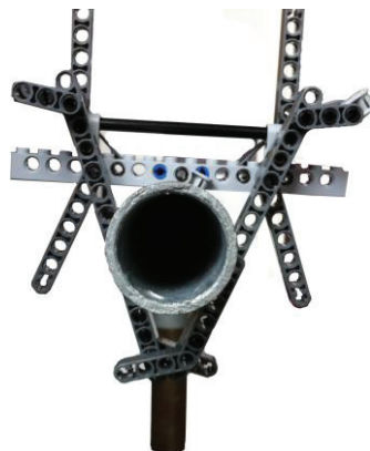
Figure 10. The claw design model gripping the projection bracket.
