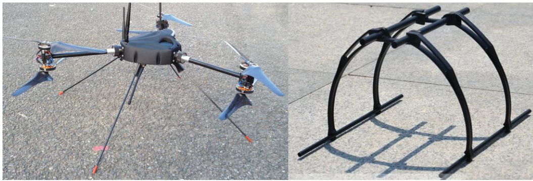
Figure 4. Landing gear types. (Left) multi point, (Right) skids.
