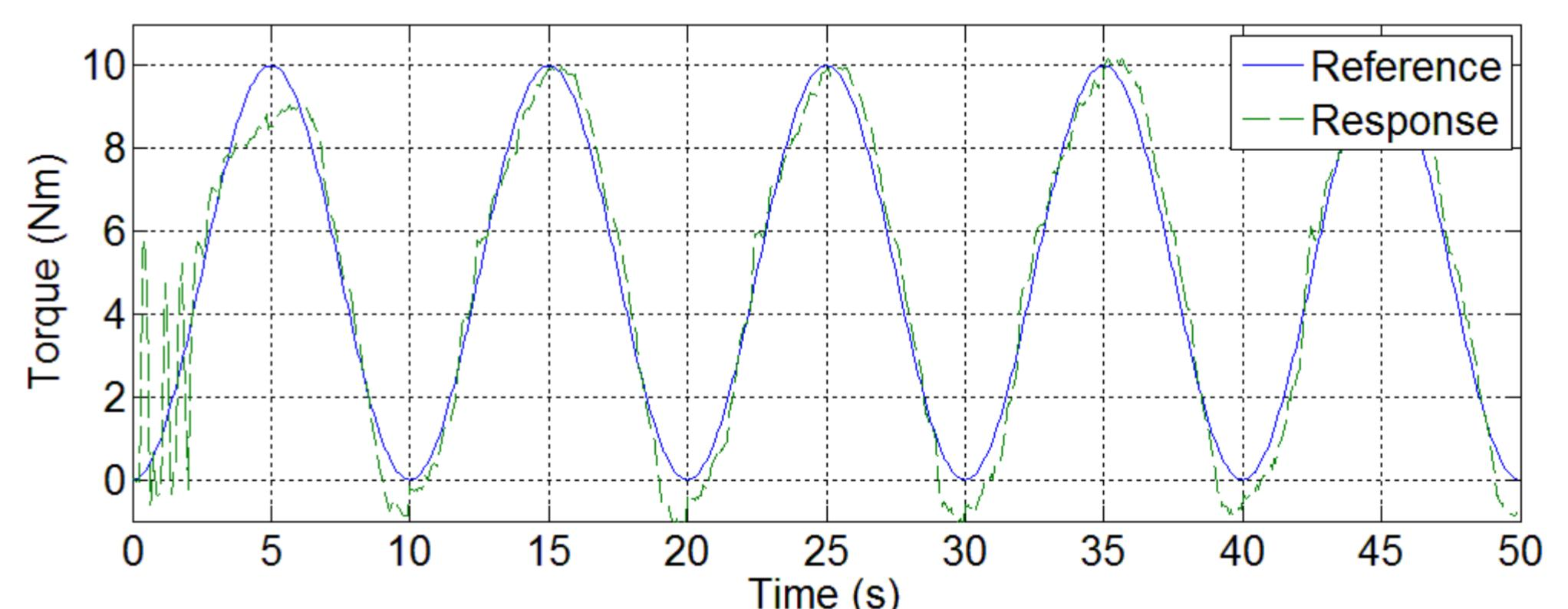
**Key Result:** The adaptive controller (EMMSAC) was able to provide superior trajectory tracking (27.5% reduction in tracking error at 95% confidence) and therefore is better suited to compensating for muscle fatigue.
