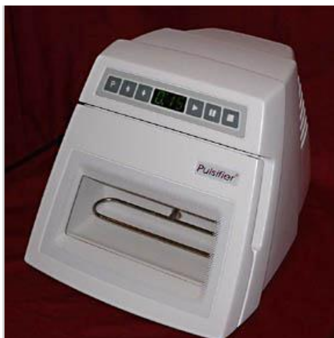
Figure 14 The Pulsifier® for recovery of bacteria from leaf samples (MicrogenBioproducts 2003)
