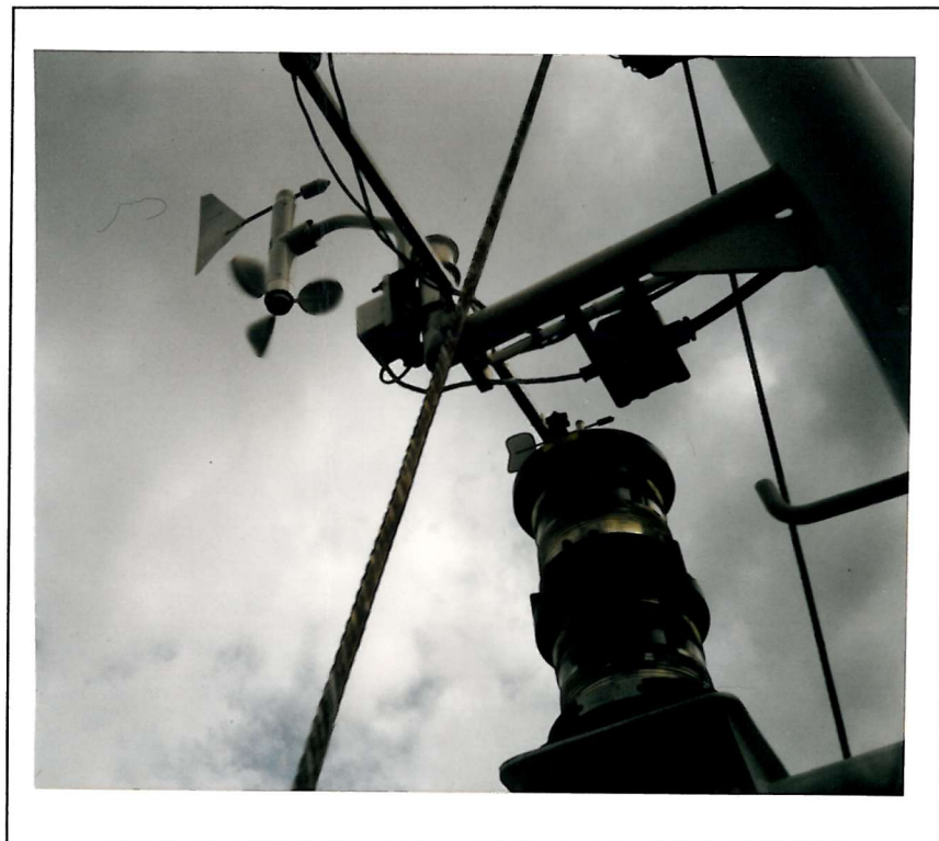
Figure 4.10 Installation of the Vector instruments cup anemometer and wind vane on the forward mast aboard the RRS James Clark Ross .
