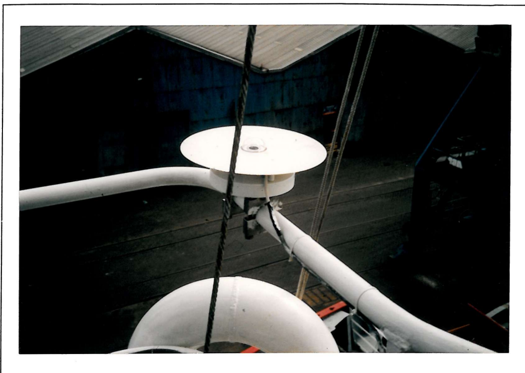
Figure 4.11 Installation of the Kipp and Zonen CM 5 pyranometer on the forward mast access platform aboard the RRS James Clark Ross .
