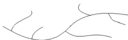
Figure 2.2: Structure of low density polyethylene
