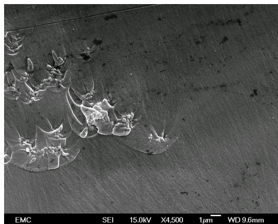
(d) EM1 epoxy system at high magnification where pinning effects can be seen.
