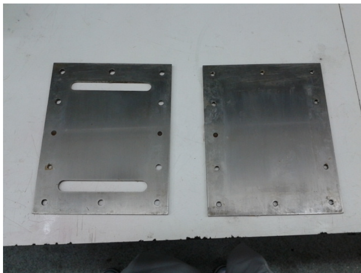
FIGURE 3.5: Gauge steel mould plates used for nanocomposite curing.
