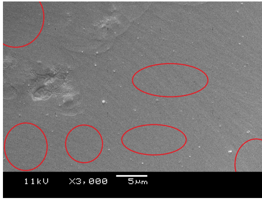
(a) Epoxy containing nanosilica after 30 min of sonication, low magnification.
