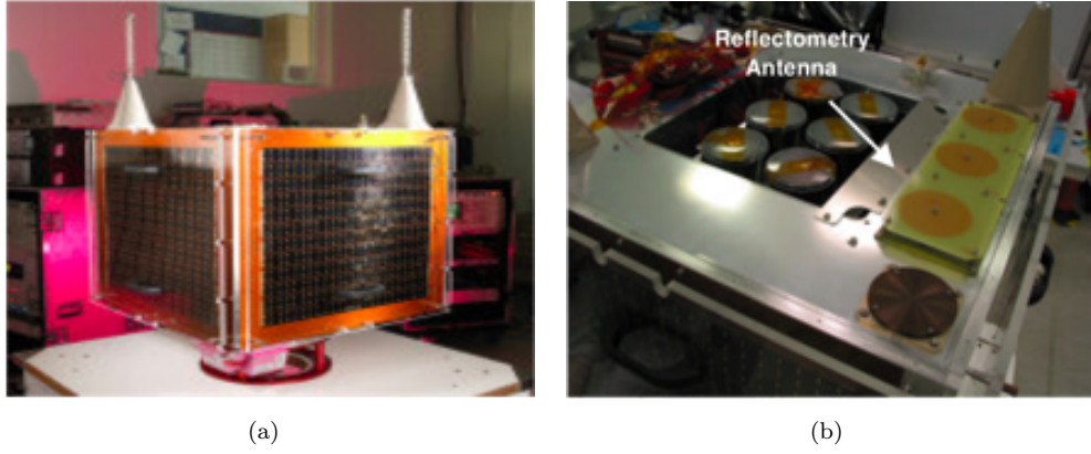
FIGURE 2.4: (a) UK-DMC Satellite in test status; (b) The UK-DMC GNSS bistatic radar antenna on the Earth facing facet [Gleason (2006)].
