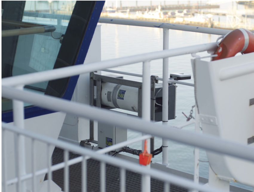
FIGURE 3.23: ISAR mounted on the starboard bridge walkway on the CpF
