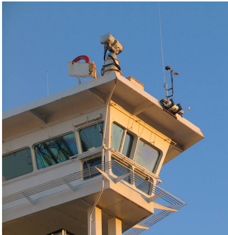
FIGURE 3.20: ISAR mounted on the starboard bridge roof on the PoB .
