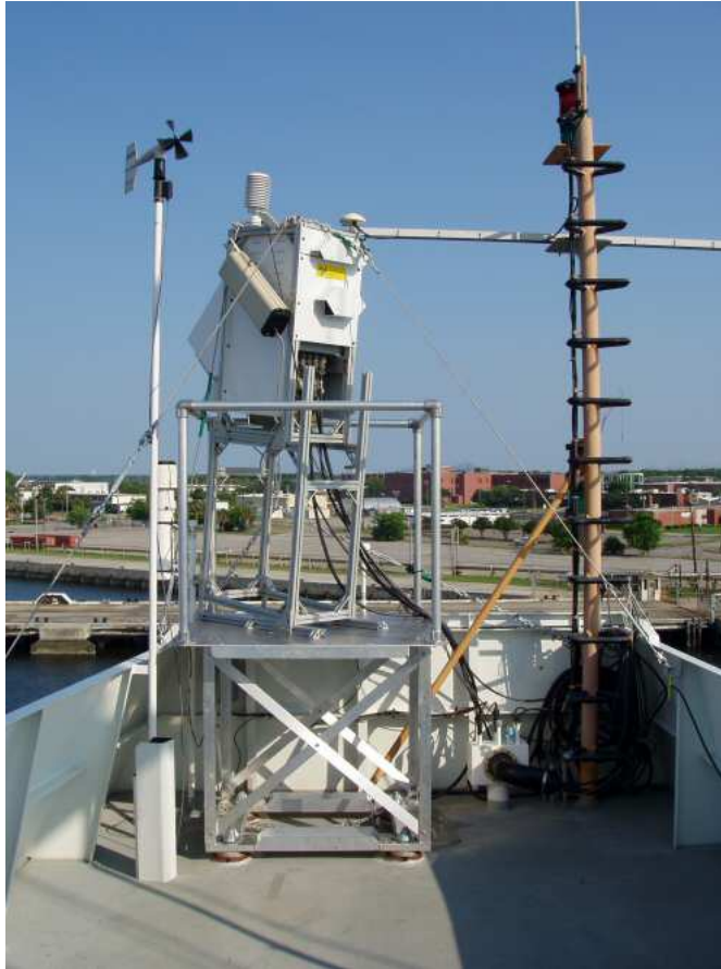
FIGURE 2.9: The CIRIMS installed on the R/V Ron Brown. From Jessup (2003).
