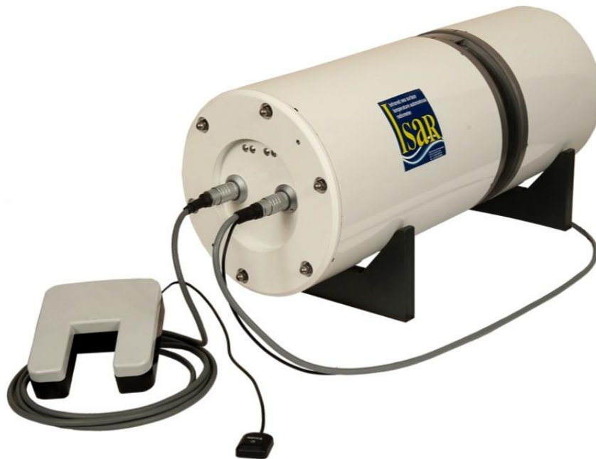
FIGURE 3.3: External view of the ISAR instrument showing the shutter open. The optical rain sensor and the GPS antennae is pictured in front of the instrument.
