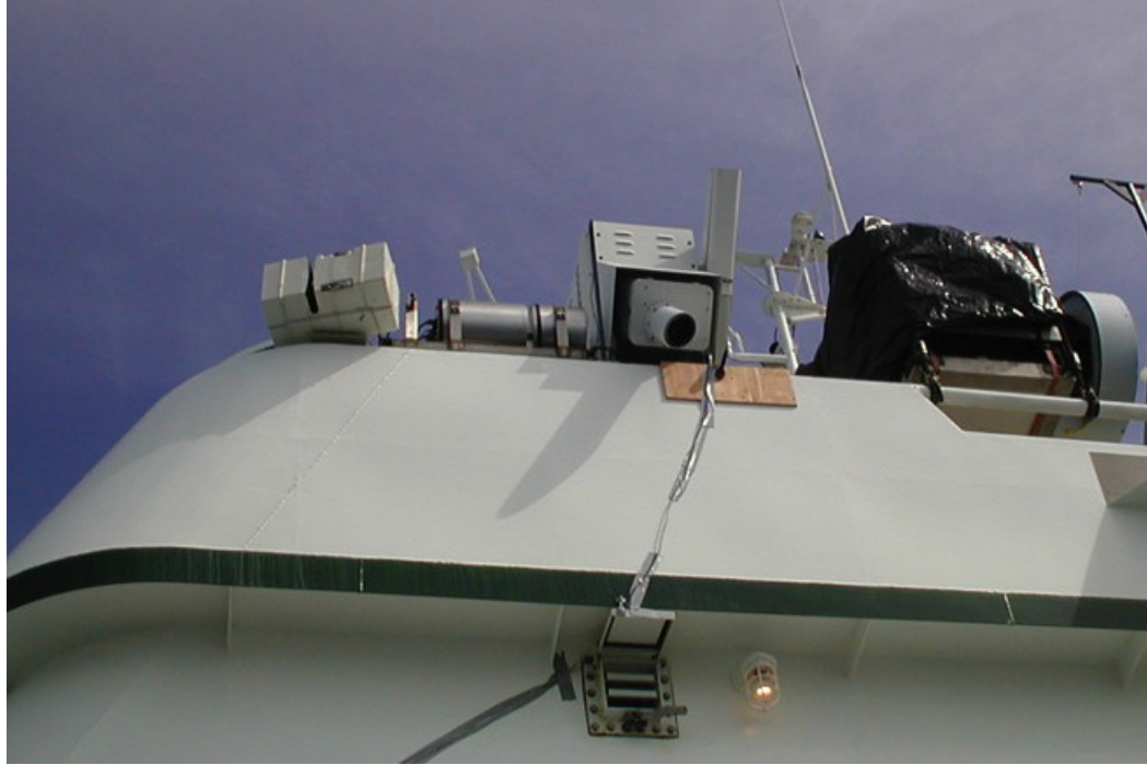
FIGURE 2.6: The Miami 2001 inter-comparison experiment. On the far right the M-AERI is visible, next is the CIRIMS , to the left of CIRIMS is ISAR 01 and far left is SISTeR . From Barton et al. (2004)
