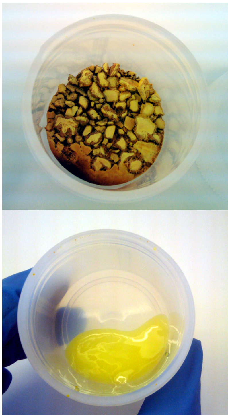
FIGURE 2.2: During \text{HF}+\text{HNO}_3 attack of large quantities of rock, insoluble fluorides can be formed. Directly after the attack they form large, polygonal grains (top pane). After further attack with \text{HCl} and Aqua Regia, the fluorides are broken down into a gel. The yellow colour of the gel indicates a significant quantity of digested rock is present within the structure of the gel. Teflon pots are approximately 3cm in diameter.
