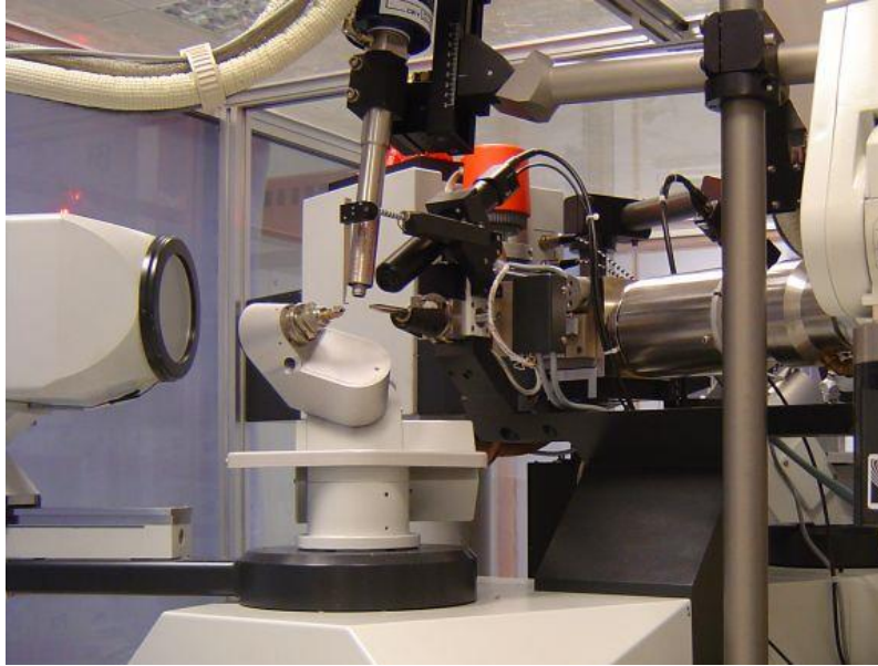
Figure 4: Image of one of two single crystal diffractometers used in this work, CCD area detector is visible on left, goniometer centre, with cyrostream, microscope and x-ray source from left to right
