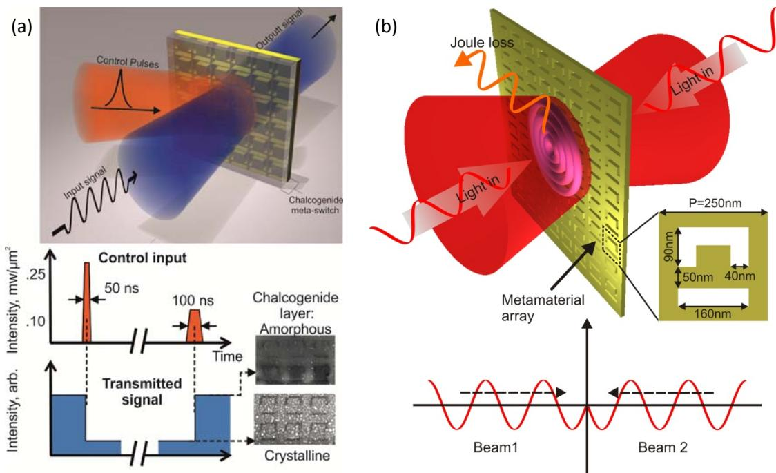
**Photonic ‘Meta-devices’:** (a) All-optical, non-volatile, chalcogenide metamaterial switch - delivers high-contrast VIS to mid-IR transmission/reflection modulation in device structures down to  $\sim 1/27$  of a wavelength thick. (b) Control of light-by-light *without* nonlinearity - two coherent light beams of arbitrarily low intensity can interact on a metamaterial of nanoscale thickness such that one beam modulates the other.
