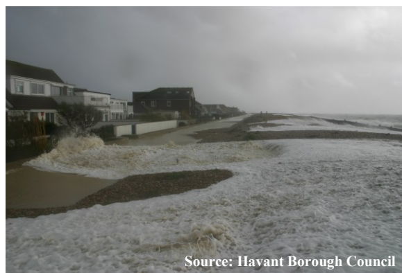
Figure 4.12 Overtopping and flooding caused by long period (swell) waves at Eastoke (Hayling Island, Havant) on 3 rd November 2005
