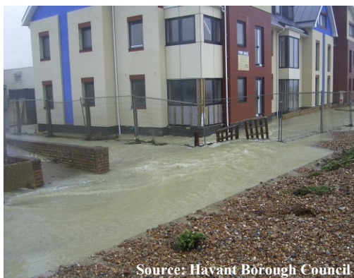
Figure 4.12 Overtopping and flooding caused by long period (swell) waves at Eastoke (Hayling Island, Havant) on 3 rd November 2005
