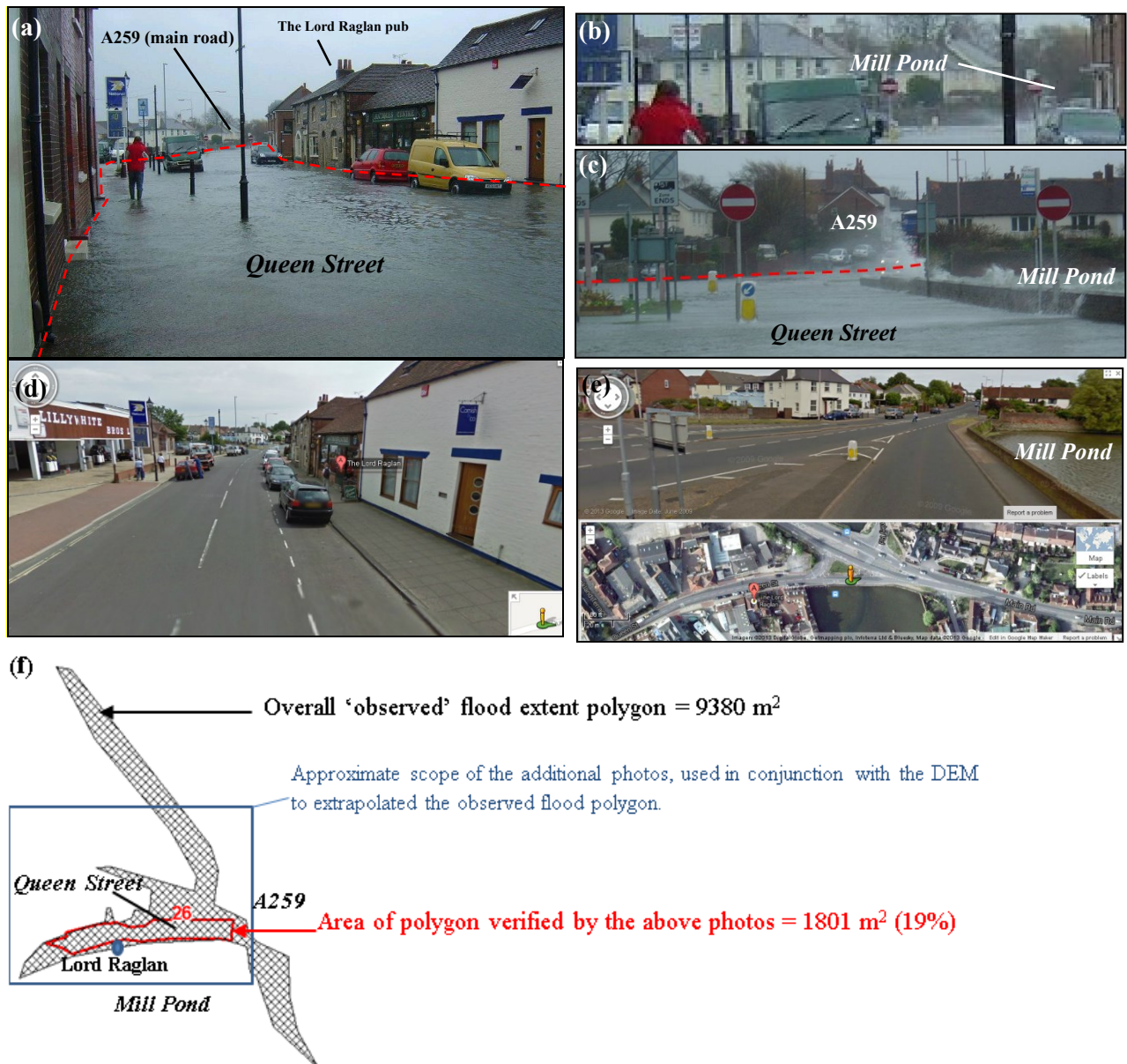
Figure 5.6 Example of utilisation of photos to approximate observed inundation extent; (a) this photo looks east along Queen Street, Emsworth (Location 26) allowing two clear reference lines along the side of the street, whereas (b) and (c) allow a closer view enabling locations to be spatially referenced to more distant landmarks, such as the intersection between the two main roads, and the wall surrounding Mill Pond. A useful tool for reference was Google Maps and Street View, as shown by (d) and (e). Figure 5.6 (f) depicts the area captured by these images in proportion to the overall flood extent – the visual interpretation (shown by the red dashed lines in the above photos) is converted to a polygon and the area is then measured in GIS. Photo sources for (a), (b) and (c): Emsworth Residents Association; source for (d) and (e) copy right Google (2013).
