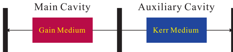
Figure 6.4: Typical structure of additive-pulse mode-locking.
