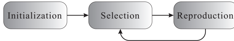
Figure 3.2: The generic blockdiagram of an evolutionary algorithm.
