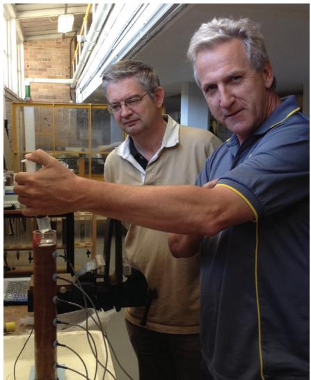
Nick Harris and Keith Smettem performing a real-time demonstration of chloride sensors mounted in a soil column.
