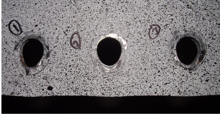
Figure 3-18: Typical deformation of beam web
