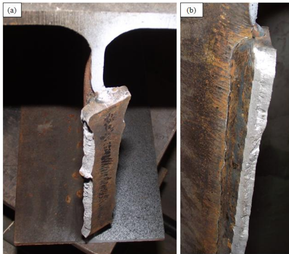
Figure 3-23: Complete failure of FEP20 showing rotation of beam web
