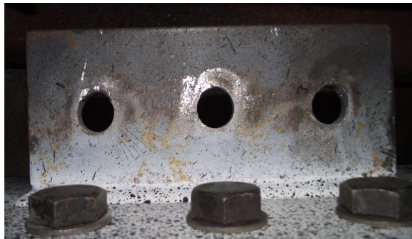
Figure 3-17: Typical deformation of fin plate
