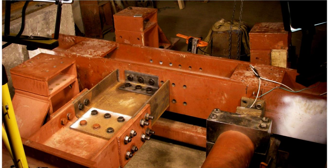
Figure 3-37: Web cleat connection in test rig prior to testing
