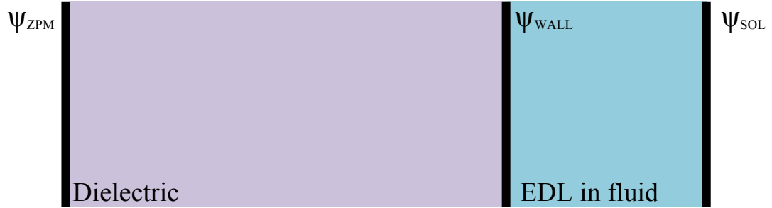
Figure 44: Illustration of the model where there is a dielectric (the channel wall) between the electrode and the solution. The model for the EDL in the fluid can be interchanged depending on the requirements.
