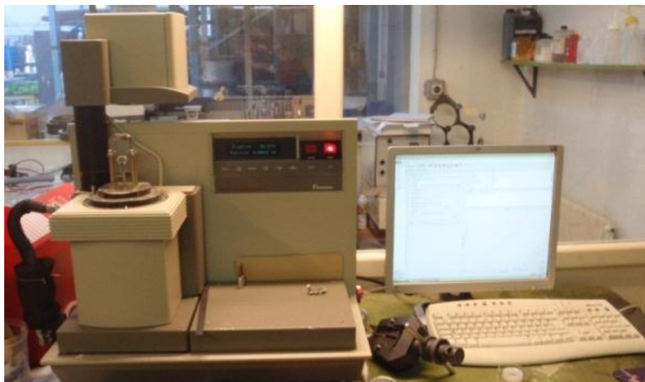
Figure 9.12: The overview of Dynamic Mechanical Analyzer DMA 2980 (IFREMER).
