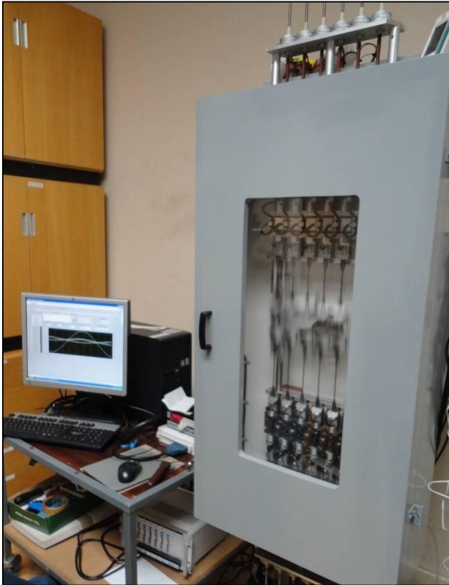
Figure 7.6: Overview of new fatigue test machine.
