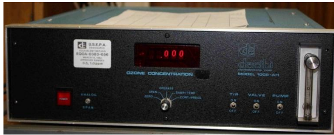
Figure 7.3: The UV Photometric Ozone Analyser used indicated a zero ozone concentration in the chamber.
