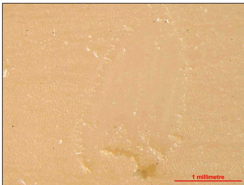
Figure 4.11: Surface for R1 (EDS19A) after scraping the shiny layer using a probe.
