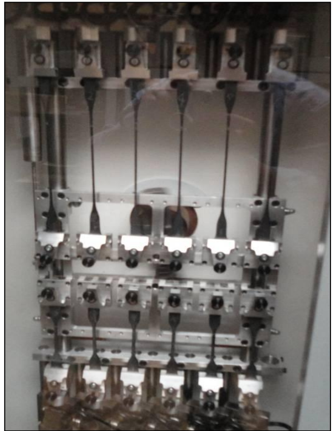
Figure 7.7: Non-relaxing fatigue test setup – Top at 265% strain and bottom at 55% strain.
