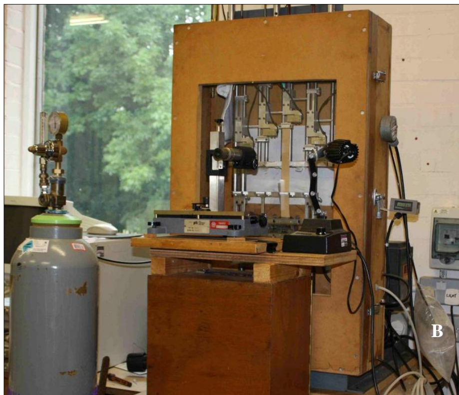
Figure 7.2: The overview of the crack growth test in an ozone free chamber. B - plastic bag.
