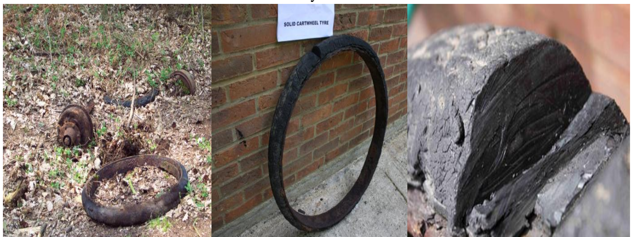
Figure 9.3: Solid rubber tyre from Bramfield Wood (left and centre) and a small portion of the tyre was taken for investigation (right).
