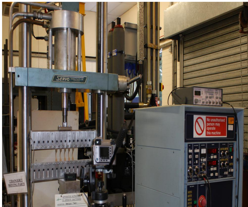
Figure 7.5: Overview of fatigue test set-up using Servotest machine at 1 Hz, with an amplitude of \pm 28.5\text{mm} equivalent to 150% strain.
