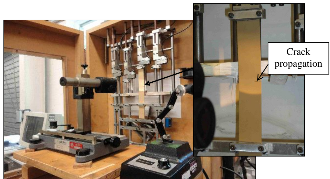
Figure 7.1: Overview of crack growth test using a simple-extension strip test piece with an edge crack at 50% strain. The test piece was installed with the testing machine in relaxed condition.
