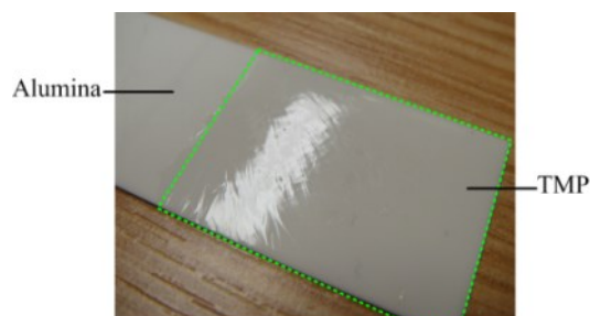
Figure 4-10: TMP paste deposited by smearing onto an alumina tile and dried at room temperature.
