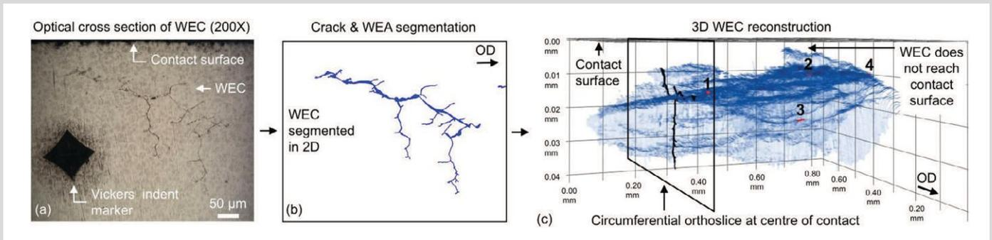
Figure 2 | Images showing process of 3D WEC reconstruction. (a) Optical image of WEC at miscellaneous slice in the circumferential plane. (b) 2D crack + WEA segmentation at slice in (a). (c) 3D WEC model of all slices in WEC model (~160 slices). No's 1-4 highlights inclusion-WEC interactions. See [4] for images and 3D crack reconstruction videos.
