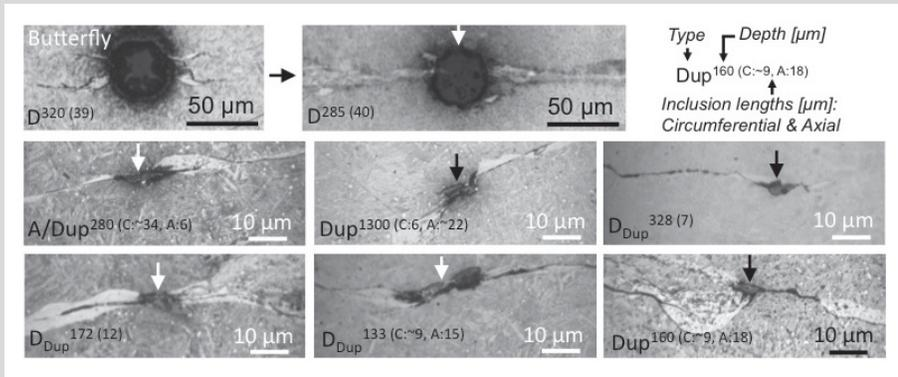
Figure 5 | Examples of inclusion-WEC interactions from the transient test gearbox bearing tests (non-hydrogen charged) and bearing from wind turbine gearbox service. Inclusion types: A (sulfide), Dup (sulfide + oxide), D (globular oxide or sulfide),  $D_{Dup}$  (globular oxide + sulfide). Images from [2].
