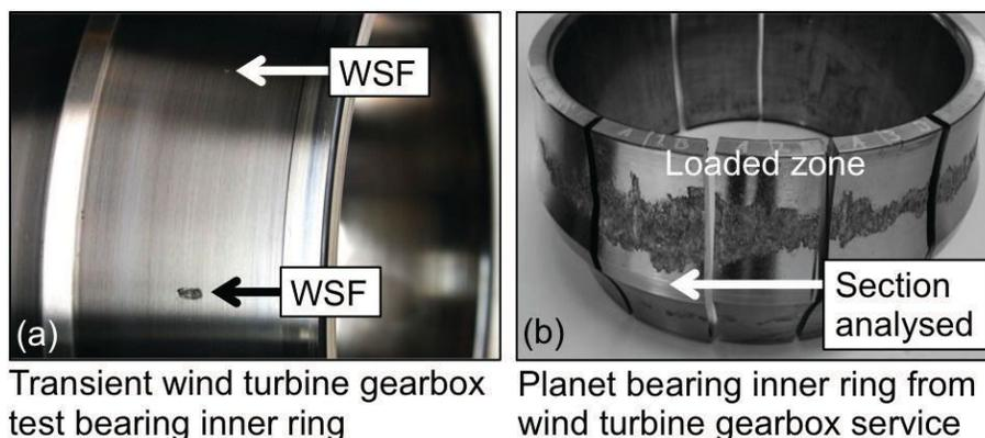
Figure 4 | Bearing inner rings analyzed by serial sectioning. (a) Two small flaking areas on inner ring raceway are apparent, where serial sectioning was conducted in their close vicinity. (b) Extensive spalling on the inner ring raceway where the serial sectioning locations were chosen at non-damaged raceway locations adjacent to the spalling. Images from [2].
