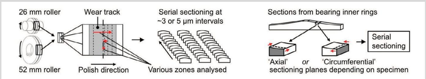
Figure 1 | Process of serial sectioning in the TE-74S test rollers and bearing inner rings.
