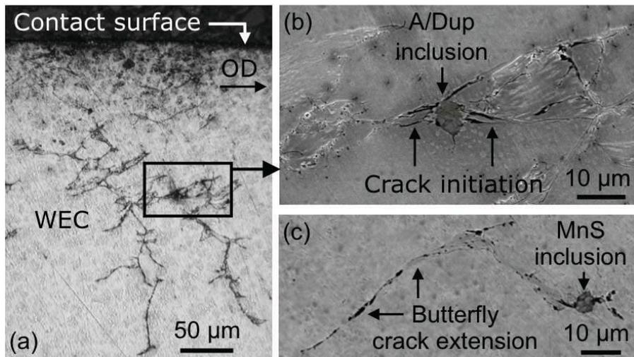
Figure 3 | Examples of inclusion-WEC interactions found in hydrogen-charged test rollers. (a) Optical image. (b) SEM image of detail in (a) showing inclusion-WEC interaction. (c) Evidence showing apparent butterfly crack propagation to WEC. Circumferential sections with over-rolling direction marked 'OD'. Images from [4].
