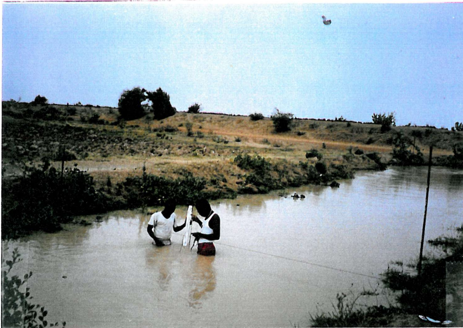
Plate 5.1 Measuring discharge in the main canal by current metering
