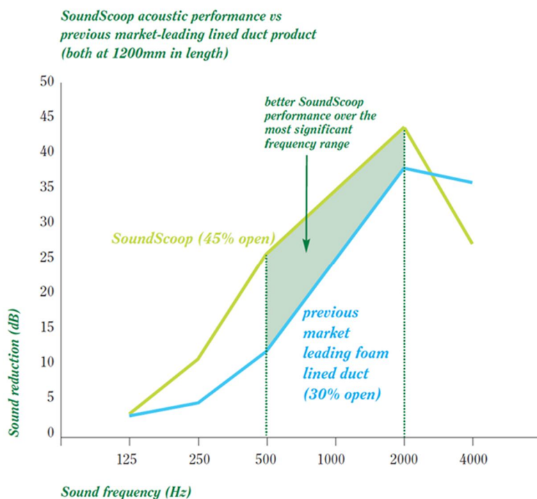
Figure 1.1: Performance of SoundScoop compared to the lined ventilation duct, obtained from SoundScoop brochure [12]
