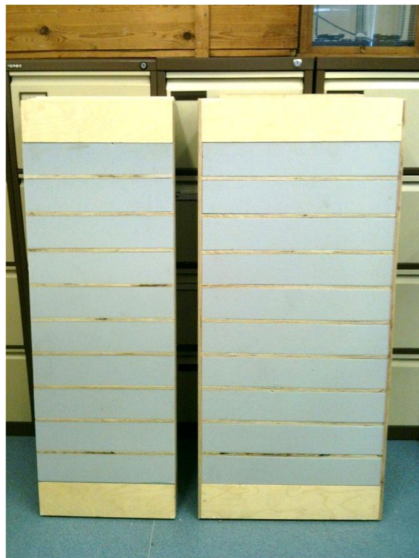
Figure 6.5: Periodically lined wall, side wall on the left and upper wall on the right
