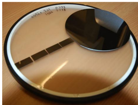
Figure 47 mounting of four silica-on-silicon chips with 100mm silicon wafer for blade dressing on the UV sensitive tape.
