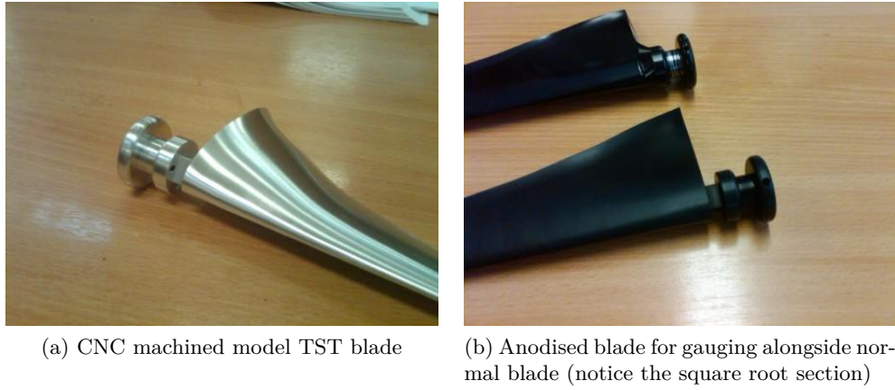
Figure 5.8: Blade root modification for strain gauging
