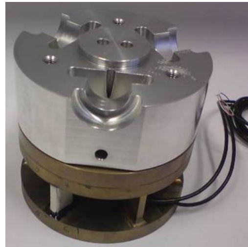
Figure 3: Thrust-Torque dynamometer and rear section of rotor hub
