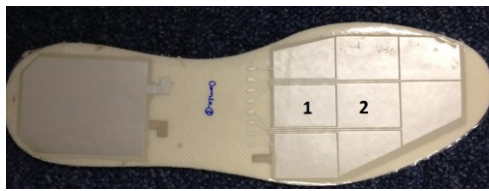
Figure 3. Top view of the printed PSI showing elements 1 and 2
