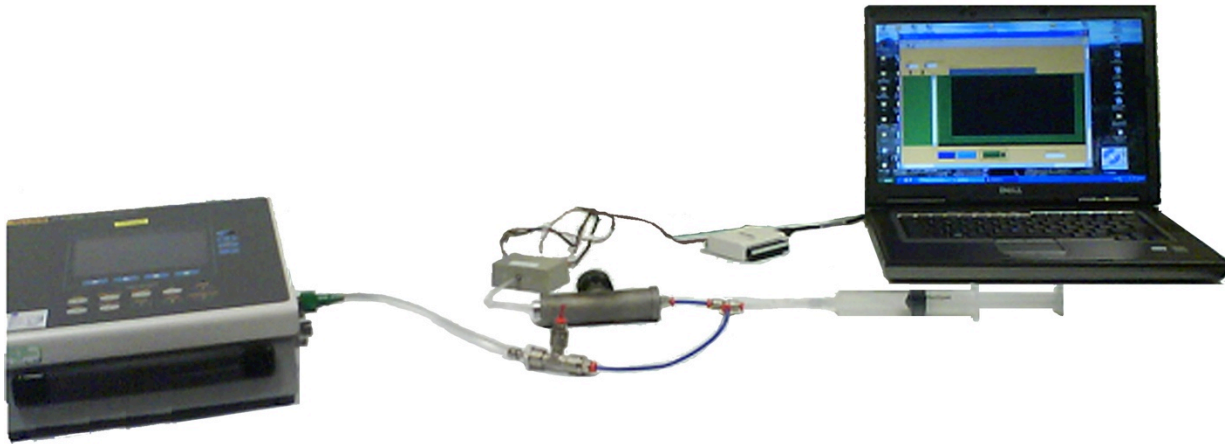
Figure 4.11 The setup for validating the pressure sensor setup using the pressure chamber and a standard calibrator
