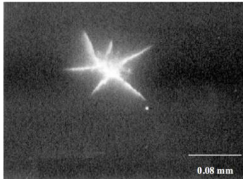
Figure 2.6: Snapshot of a Star crack under fluorescent light [43].
