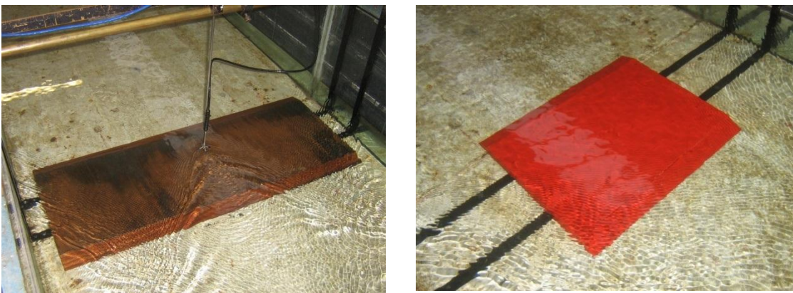
Figure 5-1: Full channel width ramp (left), half channel width ramp (right)
