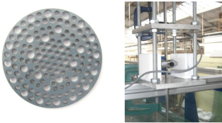
Figure 5-24: Actuator disk (left). Lever arm rig (right)
