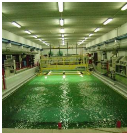
Figure 7-5: View downstream of the Ifremer water channel (left), installed mesh disk rig and ADV mounted on 3-dimensional axis (right)
