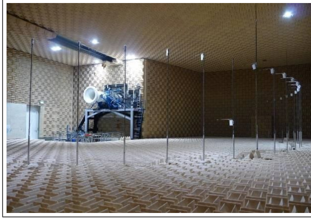
Figure 8.1 – A test rig in the process of being installed in Test Bed III at AneCom AeroTest GmbH. This inlet-side anechoic chamber has a floor area of 1000\text{ m}^2 and is 10 m high. In the foreground an array of microphones that are used for sound power measurement may be seen (see Section 9.1).
