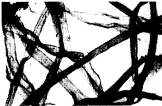
(a) Loose structure of cellulose fibres in pressboard [22]
