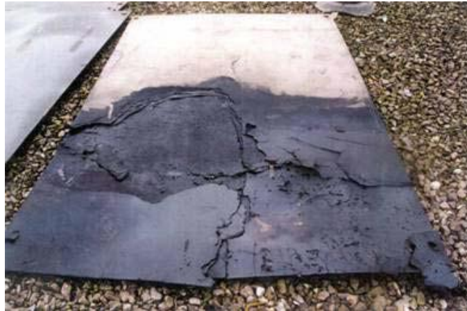
Figure 1.2: Flashover failure along barrier board [8]
