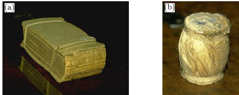
Figure 1.1: Early examples of millimeter-wave ‘metamaterials’ created by J. C. Bose [4, 5]. (a) Linear polarizer made from a book with inserted sheets of tin-foil. (b) Polarization rotator made from twisted jute.
