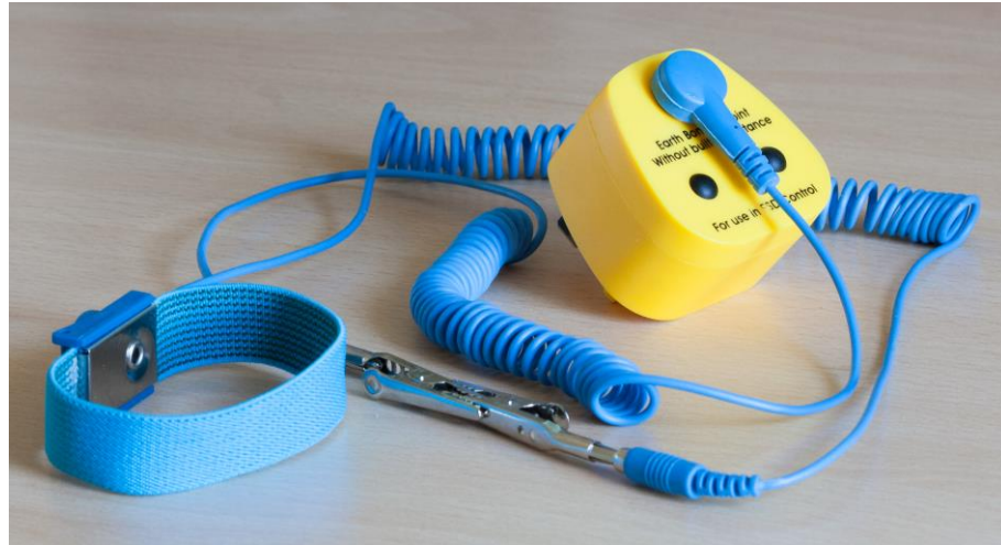
Figure 6-18: Modified earth bonding strap with unmodified earth bonding UK plug
